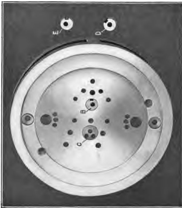
FIG. 88. — A RECESSED AND BUSHED MASTER PLATE
